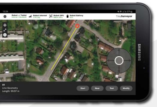
The accompanying tablet gives the operator full control of the robot as well as the parameters of the job in question. For instance, the operator can customize marking settings, apply projection shifts and adjust robot velocities directly from the tablet. Existing CSV and DXF files can be sent directly from the tablet
